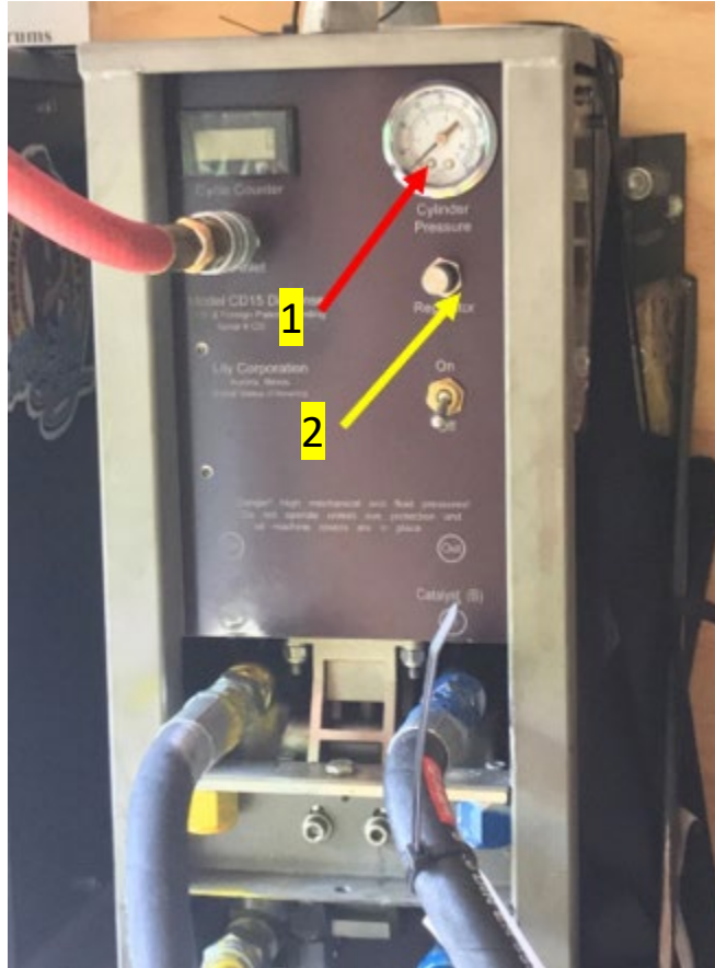
Figure 15: Cylinder gauge and regulator
