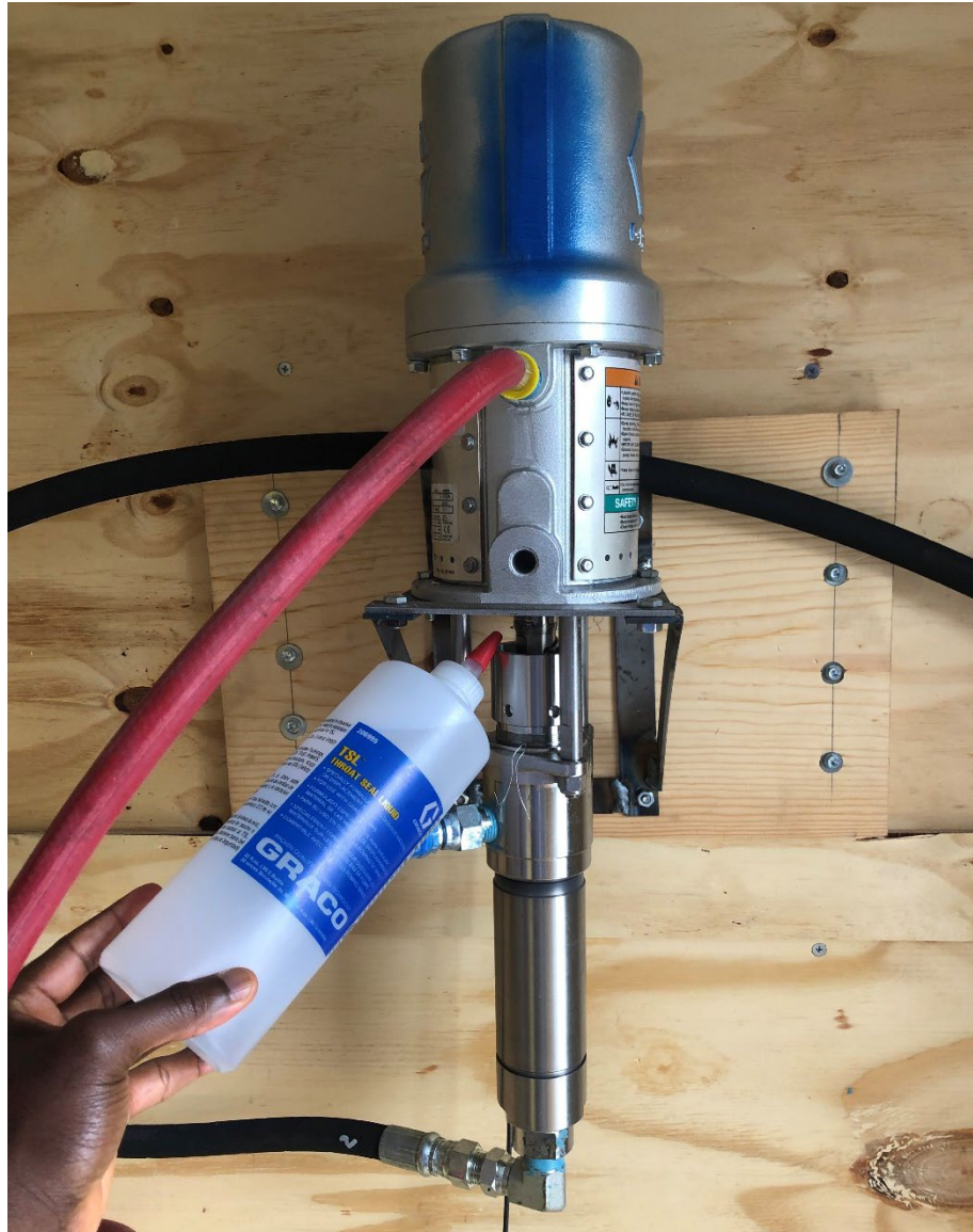
Figure 8: Filling of seal lubricant cap with Graco Throat Seal
