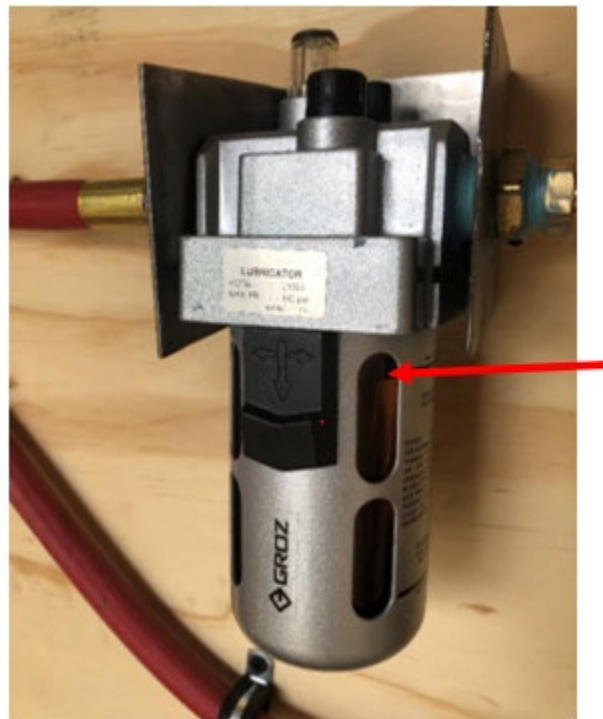
Figure 5: Oil level in lift pump container
