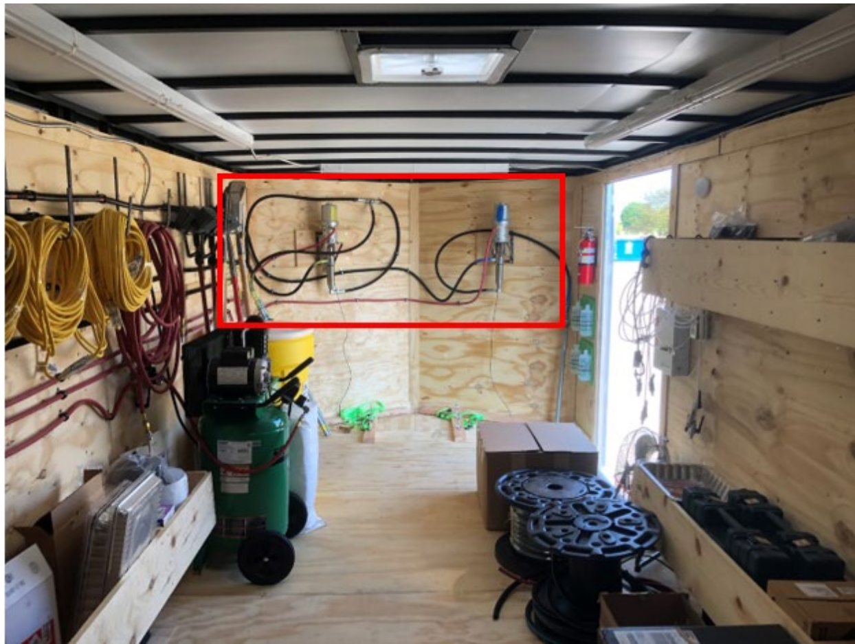
Figure 3: Location of lift pumps and oil containers
