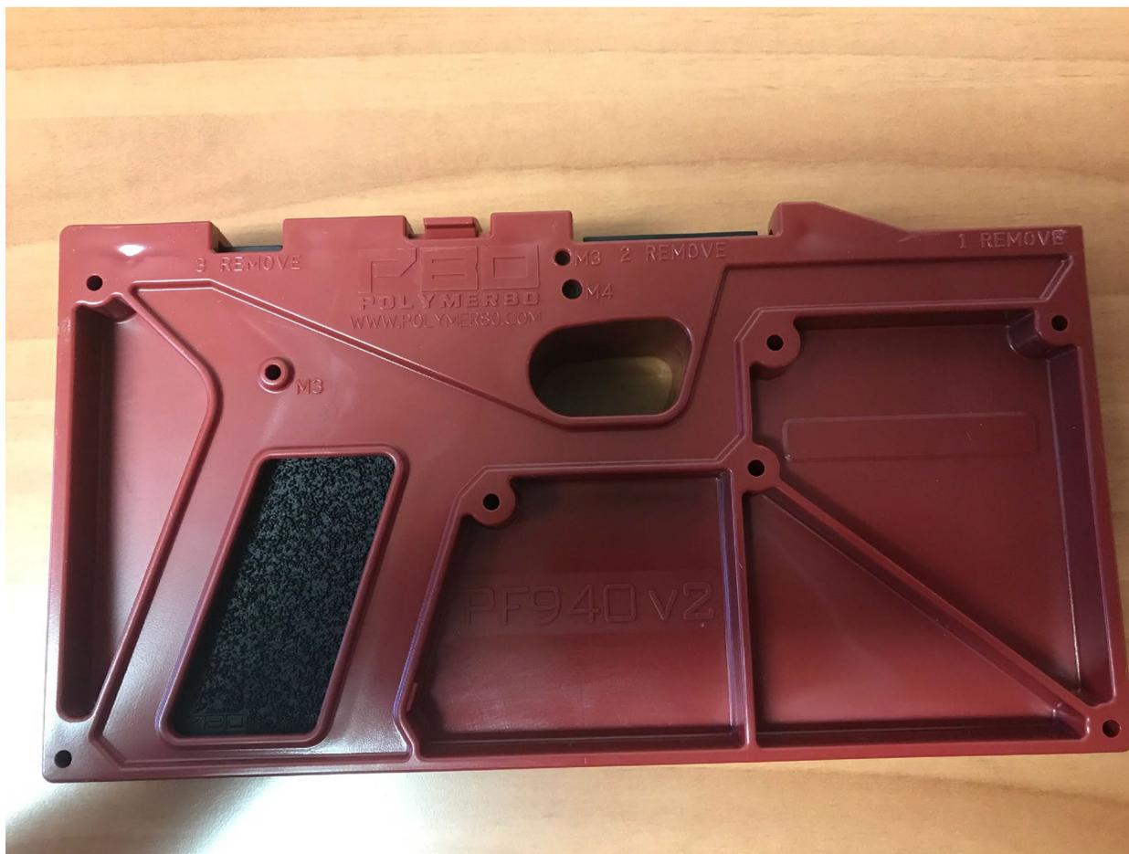
65. The unfinished handgun frame is shipped already inside the jig, and the jig itself is clearly labeled with the simple steps the consumer needs to take to “finish” the frame. The notches on the top are clearly labelled “REMOVE” – the small pieces of plastic sticking up above them
