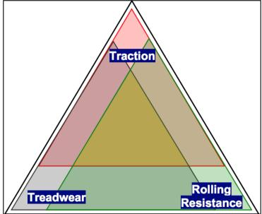
Figure 25: Magic Triangle: Traction, Treadwear, and Rolling Resistance
