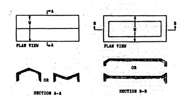
EXAMPLE C: IRREGULARLY SHAPED ROOFS WITH RECTANGULAR SHAPED SECTIONS
