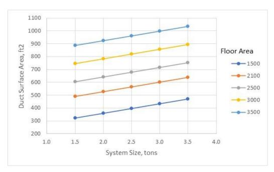
Figure 14: Duct Surface Area, 1-Story
