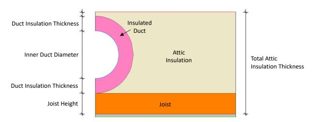
Figure 2: Insulated ducts buried within loose-fill attic insulation.
