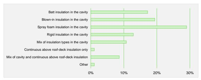
Figure 11: "How do you most commonly insulate the ceiling-roof assembly?" Participants: 93.
