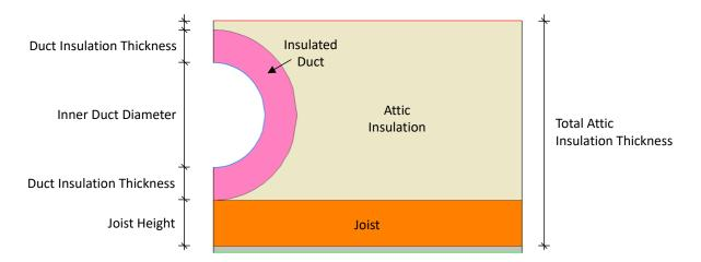
Figure 1: Insulated ducts buried within loose-fill attic insulation.
