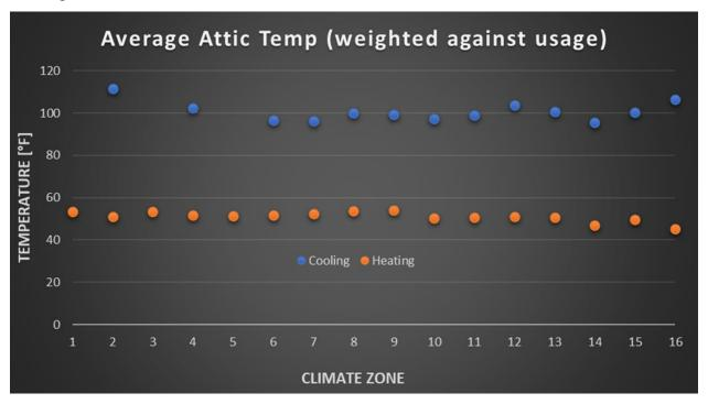
Figure 13: Average attic temperature used to calculate effective R-values of buried ducts.
