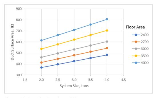
Figure 15: Duct Surface Area, 2-Story
