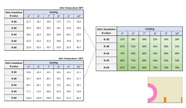
Figure 5: Impact of assumed attic temperature (80°F compared to 130°F) on effective R-values of ducts. The right-hand table presents the difference in R-value between the two cases in percent.
