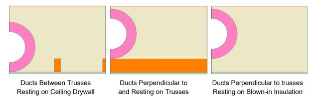
Figure 4: Simulation cases to represent location of ducts buried in insulation.
