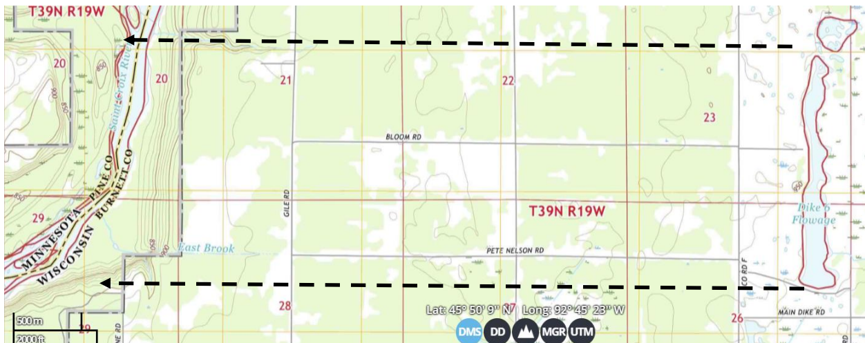
Figure 5. Illustration of simplified groundwater flow model west of Dike 6 flowage. A rectangular groundwater flow system is assumed, originating at Dike 6 flowage and extending to the St. Croix about 3 miles away. The flow system has a width of 1.2 mi.
