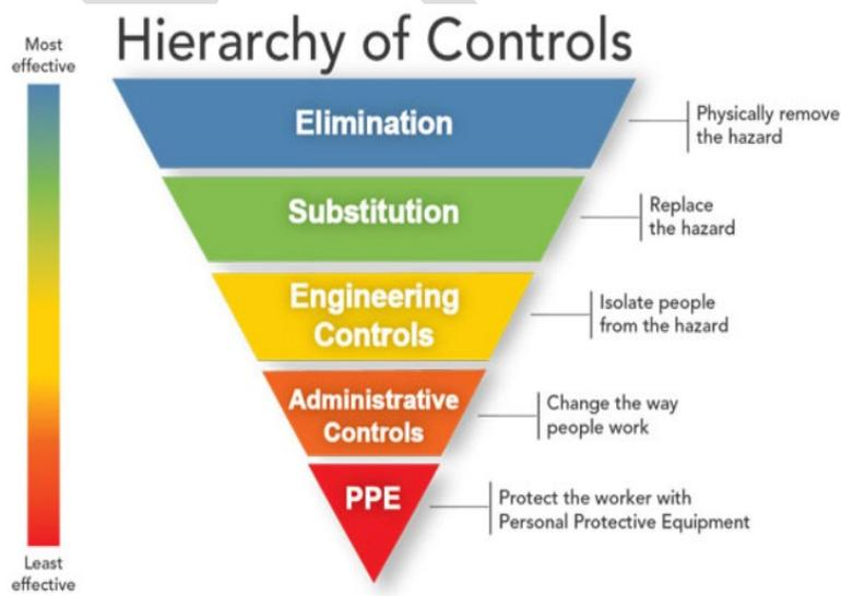
**Figure B:** Adaptation of the Hierarchy of Controls for Controlling Environmental Heat as a Hazard at Schools
