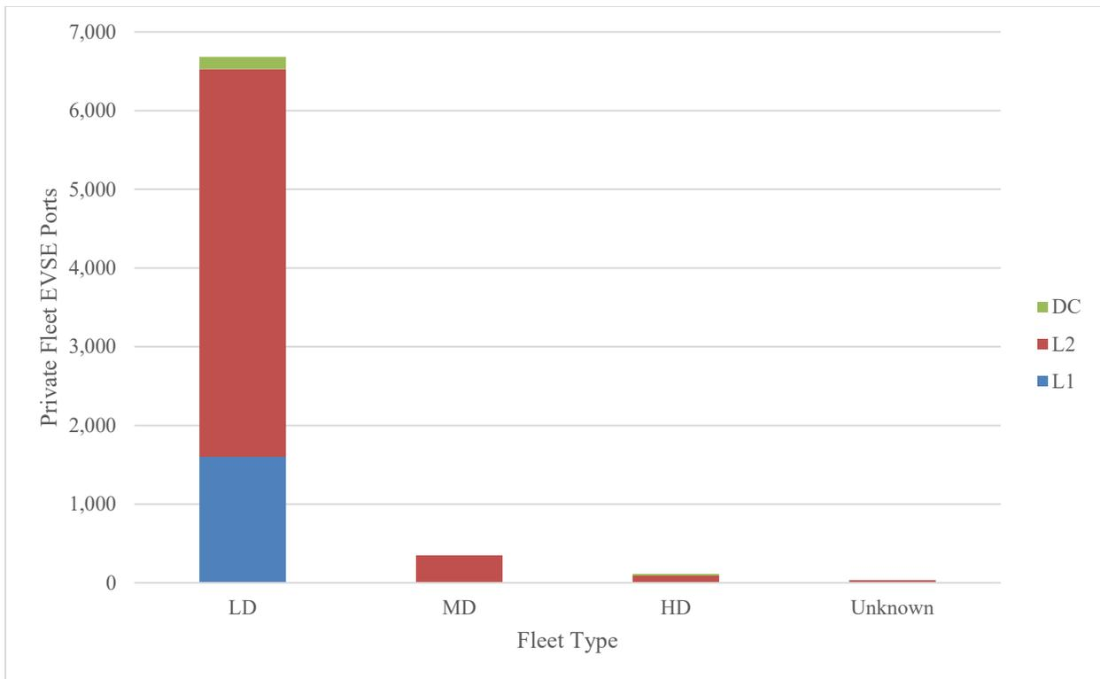
**Figure 19. Breakdown of private fleet EVSE ports by fleet type and charging level in Q1**
