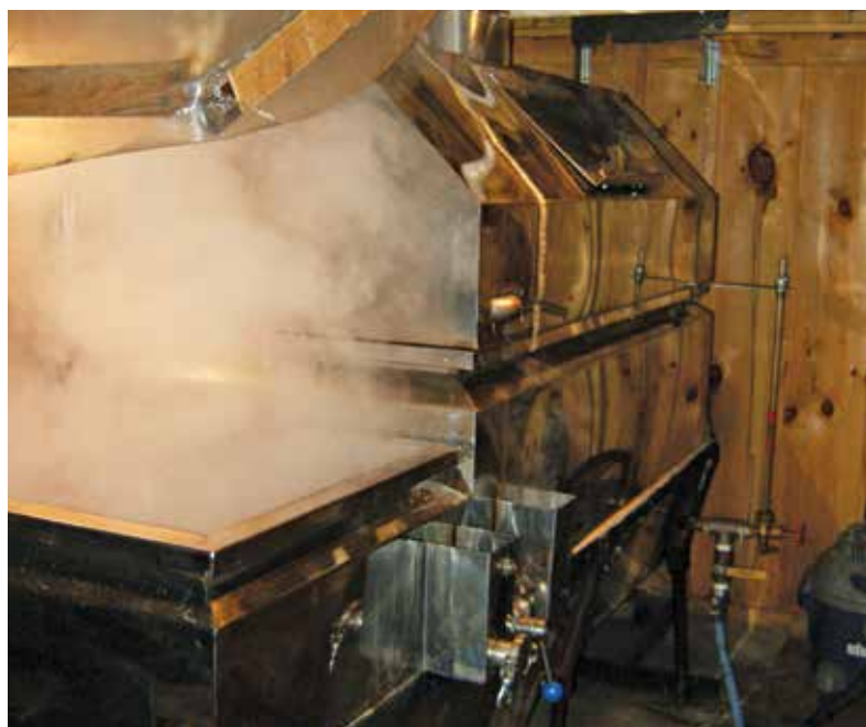
Inside a sugar house, a boiler concentrates the sap by removing water as steam.
