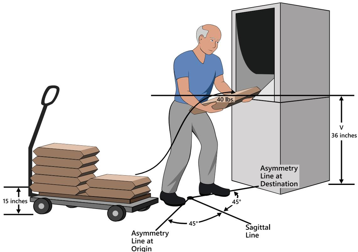
Figure 11: Loading Bags Into Hopper, Example 3
