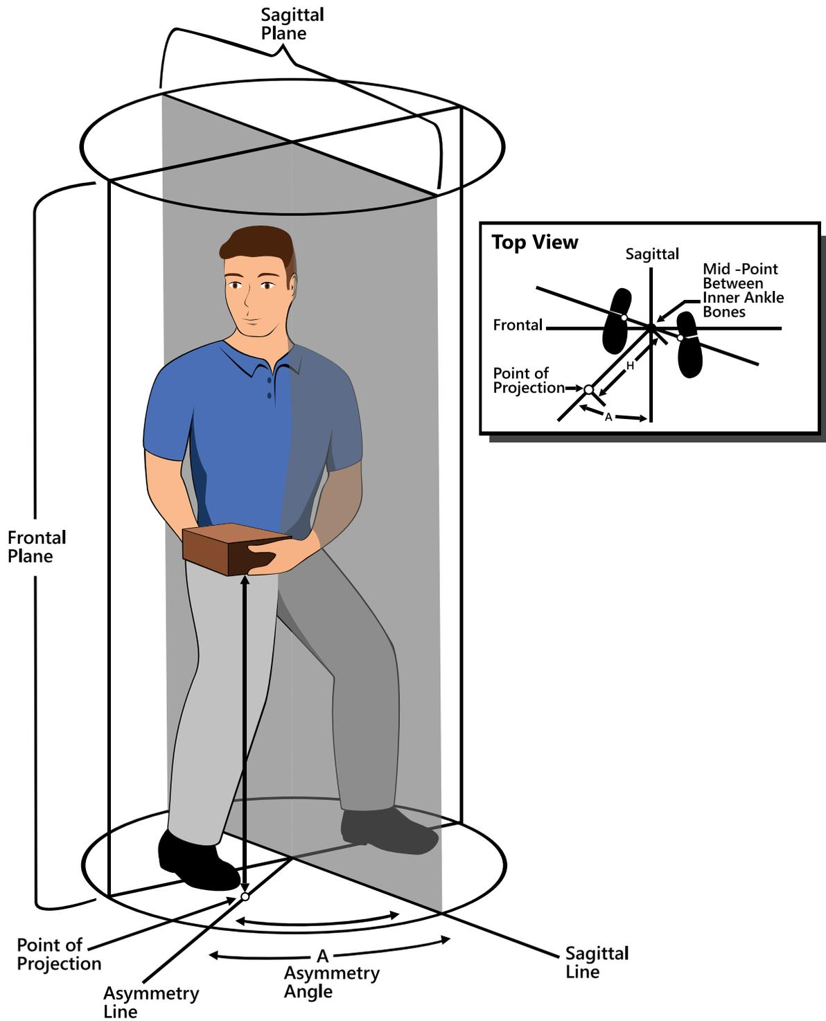
Figure 2: Graphic Representation of Asymmetry Angle (A)
