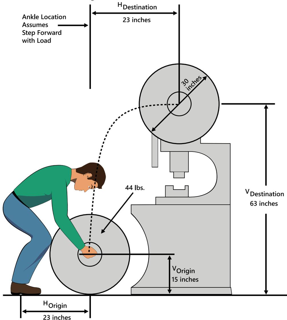
Figure 5: Loading Punch Press Stock, Example 1
