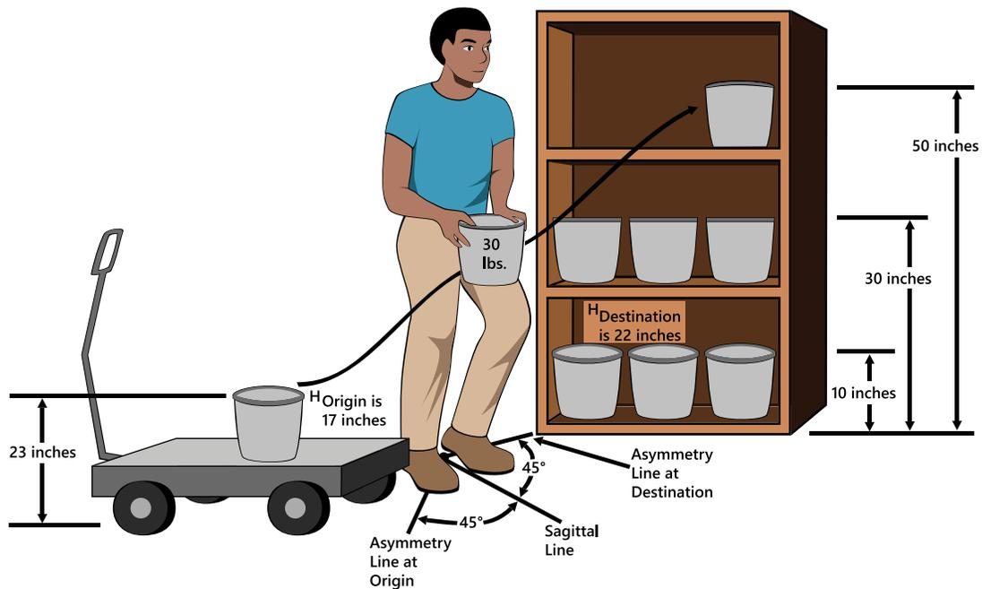
**Figure 23: Handling Cans of Liquid, Example 8**
