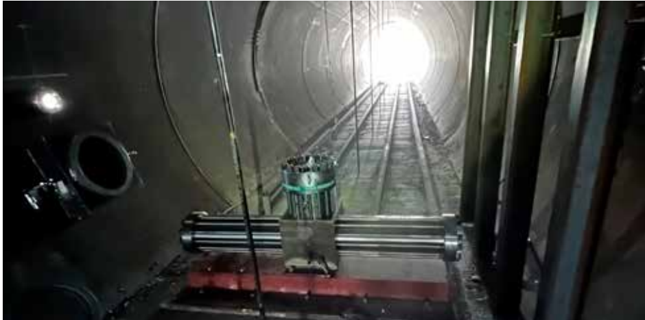
Experimental setup for HyTunnel project, showing internal view of the 70m test tunnel with the hydrogen release vessel and ignition instrumentation in the foreground, sensor arrays down the centre of the tunnel to monitor progression of the release.
