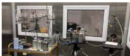
Close-up image of multiple impinger air samplers used for sampling during air cleaner testing
