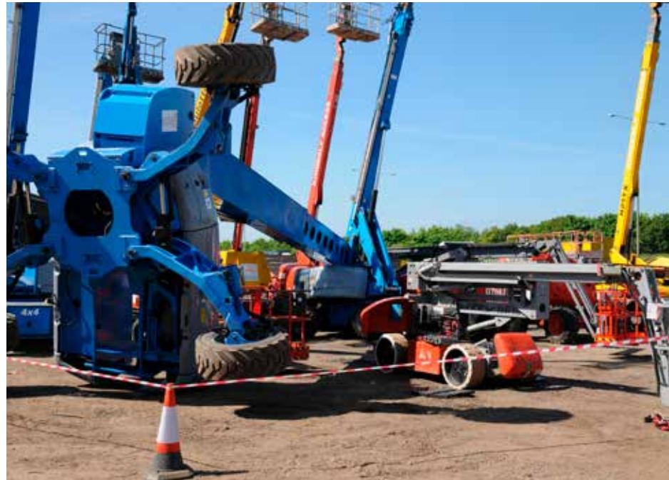
Position of MEWP following toppling incident with the boom falling outside the confines of the premises, onto the M25
