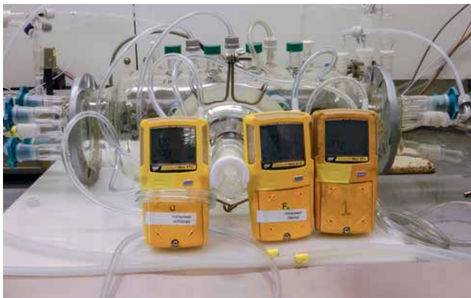
Flammable gas monitors being tested in the HSE's Science and Research Centre Standard Atmosphere test facilities
