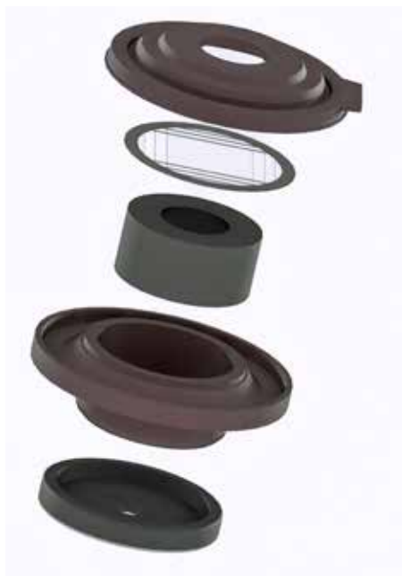
Exploded design for modified filter cassette holder for respirable sampler
