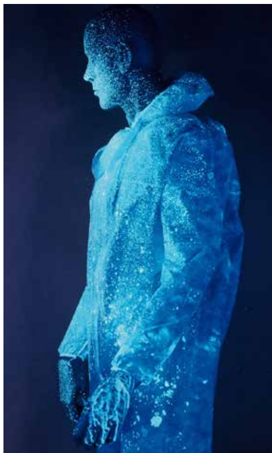
The deposition of fluorescent-labelled MWF onto the body of a test manikin after operation of a compressed airgun
