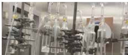
Close-up image of multiple impinger air samplers used for sampling during air cleaner testing
