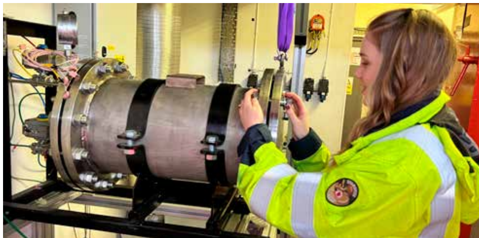
HSE scientist Gemma Howard with the equipment she designed for experiments to drive a nail into a battery sealed inside a gas-tight pressure vessel
