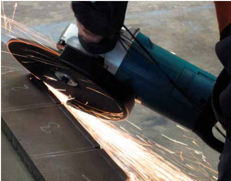
An angle grinder being tested for noise and vibration
