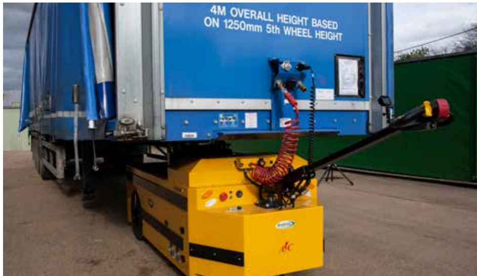
Pedestrian-operated trailer mover undergoing HSE testing
