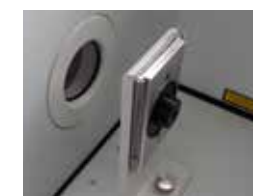
Modified cassette and holder in a portable FTIR
