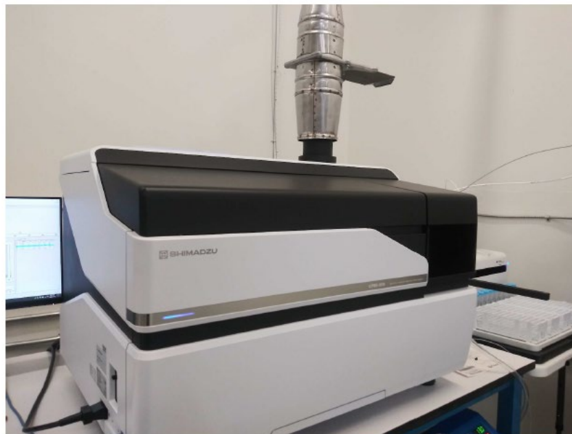
Figure 1. Inductively Coupled Plasma Mass Spectrometer (ICP-MS) from Shimadzu Scientific. Picture taken at Confidence Analytics in Redmond Washington on July 6th, 2020. The unit can test up to 20 samples per hour for heavy metals analysis. This unit alone has enough capacity to test over 10,000 samples per month, giving it plenty of capacity to meet future demand. Confidence Analytics will be submitting a validation report to the RJLee Group in the coming weeks.
