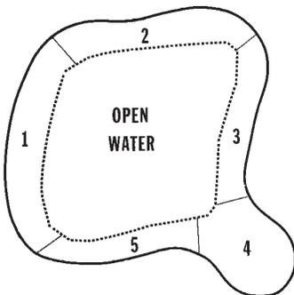
Before you apply the chemical to a treatment zone, you need to know the area (acres). To determine the area, measure the length and width in feet. Multiply the length by the width and divide by 43,560 (the number of square feet in one acre)
