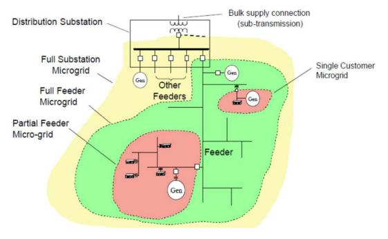
Figure 1. Microgrid Scale Variations
