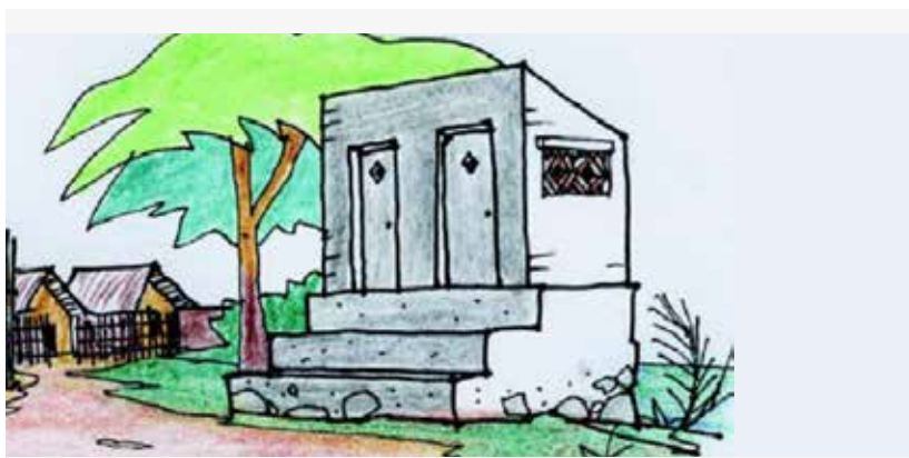
IMAGE 14. Rainwater and flooding. Rainwater harvesting can be done by using jars and pots; they need to be covered afterwards to avoid mosquito larvae. Elevated latrines reduce the risk of water-borne diseases, and epidemics in times of floods.
