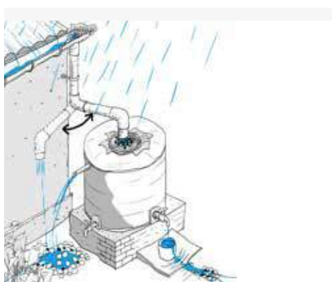
IMAGE 14. Rainwater and flooding. Rainwater harvesting can be done by using jars and pots; they need to be covered afterwards to avoid mosquito larvae. Elevated latrines reduce the risk of water-borne diseases, and epidemics in times of floods.
