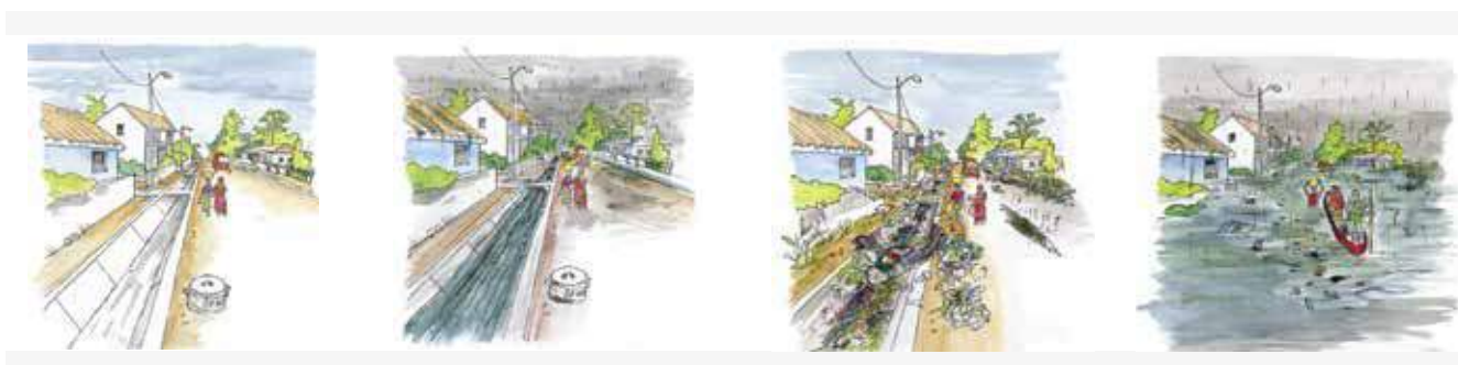
IMAGE 17. Clean drainage system to avoid floods. Often drains are not maintained and become waste disposals. The system will not be able to evacuate rainwater if waste dumping is blocking natural drain pattern, hence, generating a disaster. Credit of all illustrations: Eduardo Feuerhake
