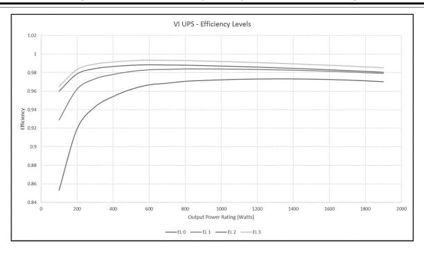
Figure IV-2 Graphical Representation of VI UPS Efficiency Levels
