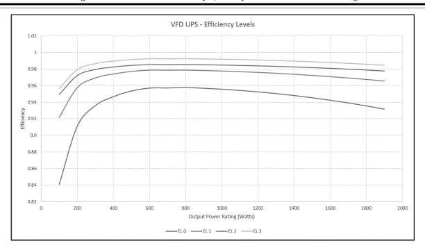
Figure IV-1 Graphical Representation of VFD UPS Efficiency Levels
