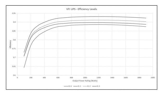
Figure IV-3 Graphical Representation of VFI UPS Efficiency Levels
