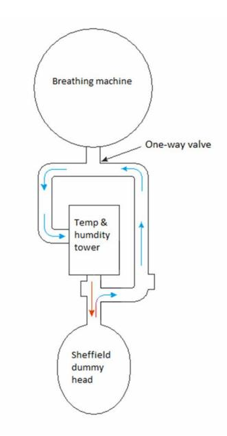
Figure 1 – Simulated wear test setup
