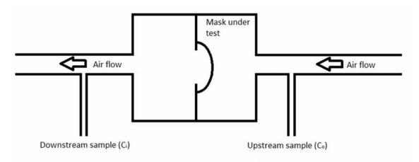
Figure 2 – Filter penetration test setup
