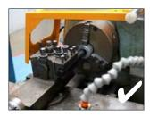
This technique combines the tool post with the holding device. The emery cloth is wrapped around the holding device and held in a boring bar holder in the tool post (see video demonstration at www.hse.gov.uk/ engineering/lathes.htm). This method is used for internal deburring. Work is simple to set up and significantly reduces the risk.
