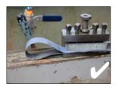
The tool post is used to clamp and hold a looped strip of emery cloth in place during application (see video demonstration at www.hse. gov.uk/engineering/lathes. htm). This method is for external deburring work only. It almost entirely eliminates the risk of injury.
