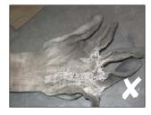
The wearing of gloves increases the risk of entanglement and is never acceptable near rotating parts of machinery such as manual metal working lathes The wearing of loose, baggy clothing, long hair and jewellery all increase the risk of entanglement.
