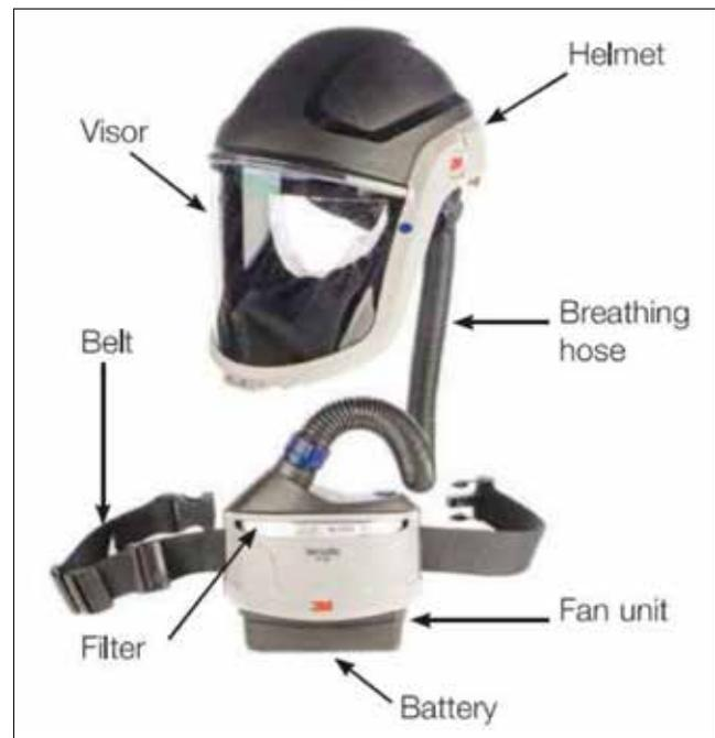
Figure 8 Powered respirator with hood/helmet
